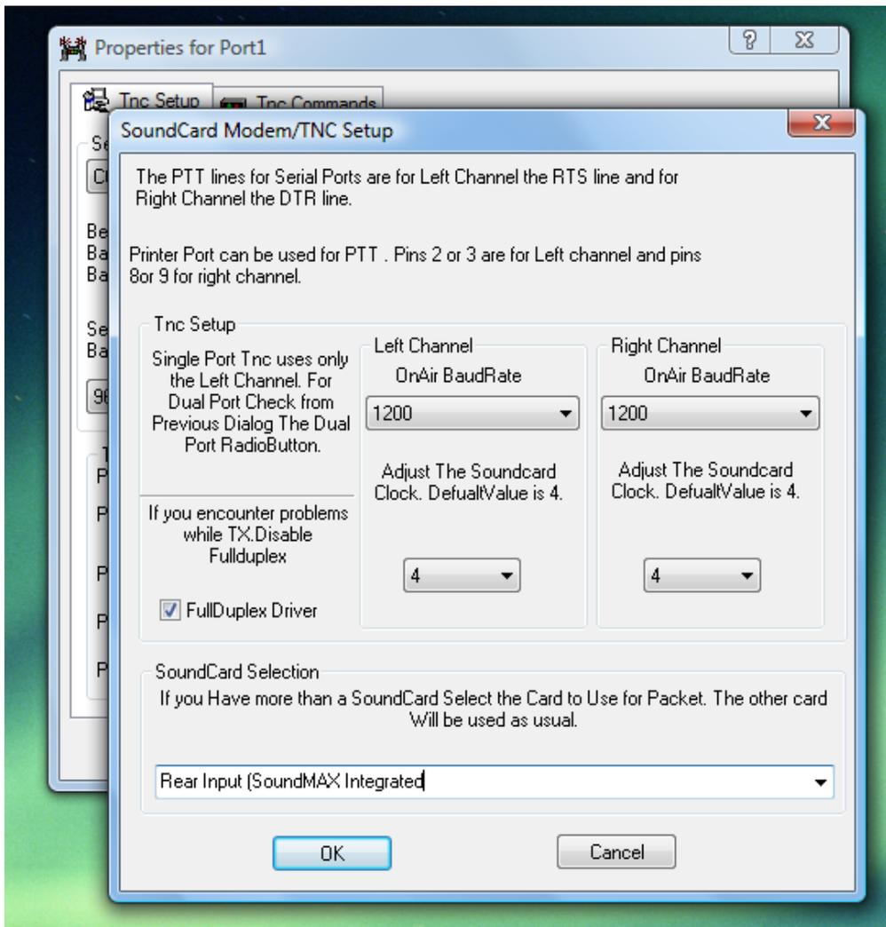
Figure 4 - Soundcard Modem/TNC Setup
